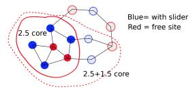
Remove recursively blue sites with less than 2 links and red sites with less than 3. What remains is the "2.5-core". Then add recursively blue sites with one link to the core, and red sites with 2. One gets the "2.5 + 1.5-core".
