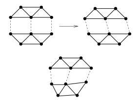
Top: a non generic realization; Laman theorem does not apply. Bottom: a generic realization of the same graph.
