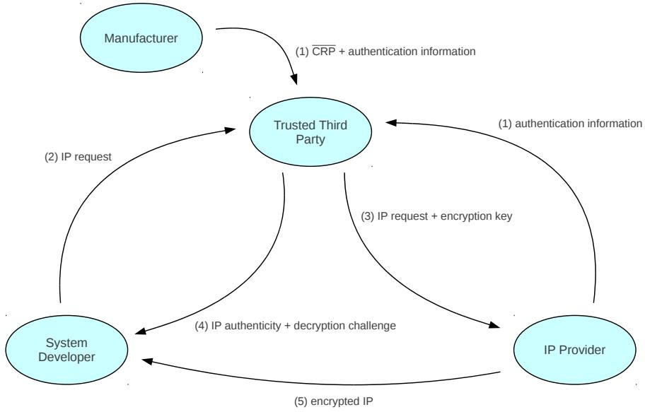
**Fig. 4.** Simspon et al.’s IP protection protocol based on PUFs.
