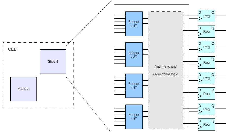
**Fig. 1.** Xilinx Configurable Logic Block and detailed Slice (dashed registers are optional, they can be bypassed).
