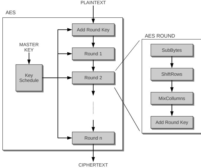
**Fig. 3.** AES encryption block diagram.
