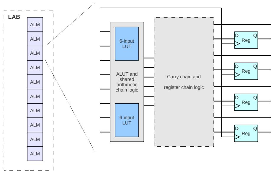
**Fig. 2.** Altera Logic Array Block and detailed Adaptive Logic Module.
