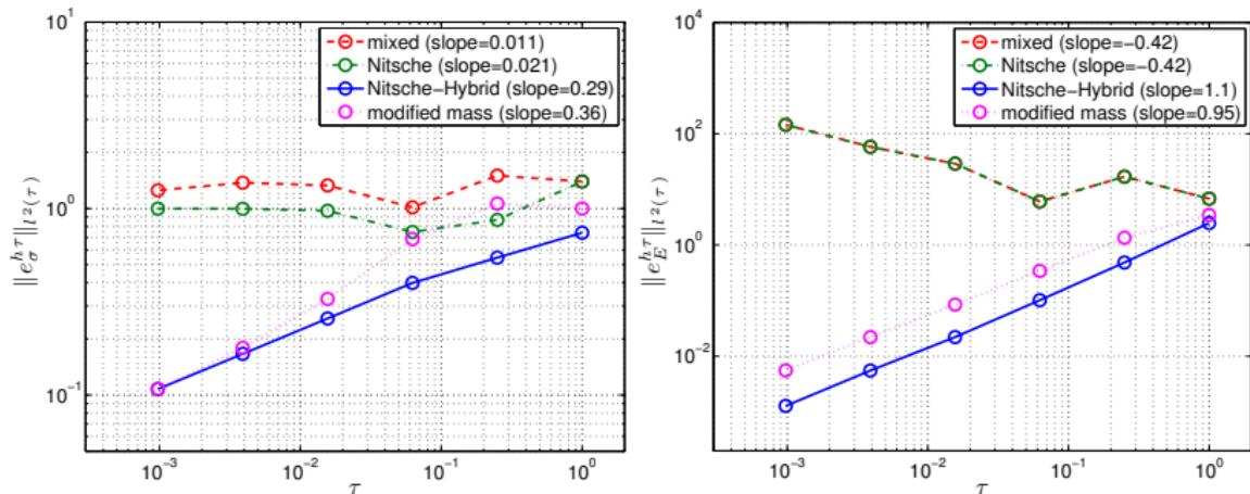
Error curves for the contact pressure  $\sigma_C$  and for the energy  $E$ .
