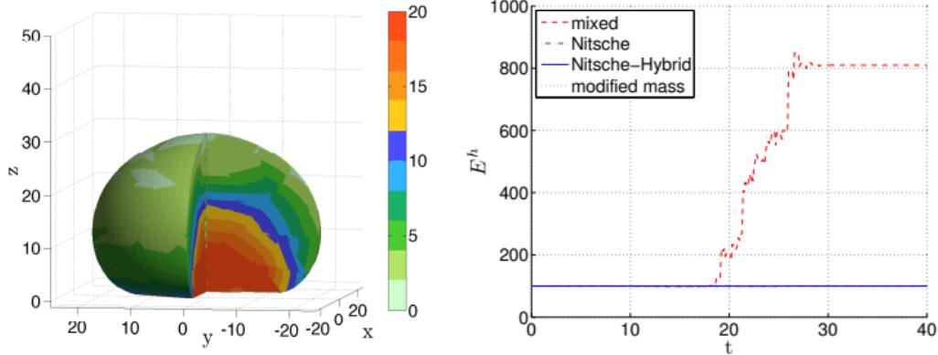
Deformed configuration and von Mises strain at  $t = 18$ , for Nitsche-Hybrid. Energy  $E^h$  for different methods.
