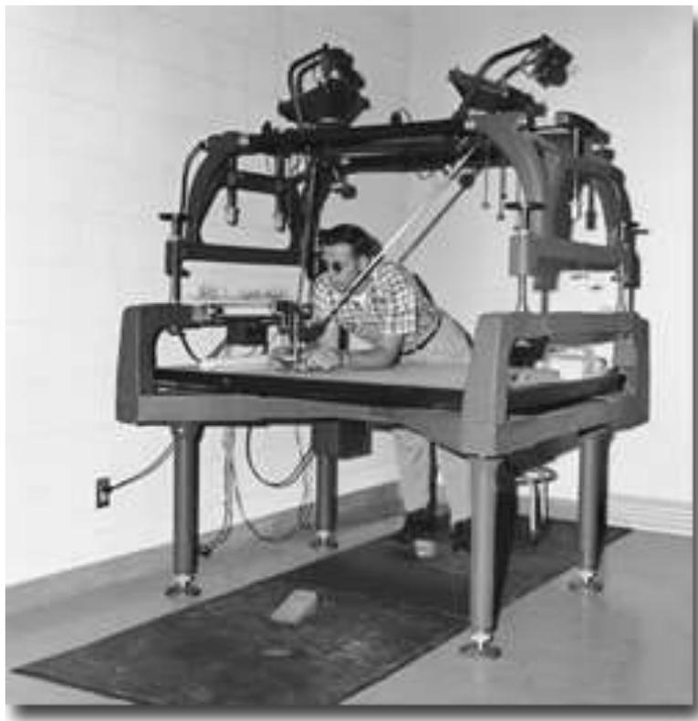
Kelsh Plotter - Initial machine used to launch the District's "in-house" photogrammetric mapping program in 1957.
